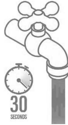
**STEP 2: After 30 seconds**, while the water is flowing place the sample bottle under the fixture and fill the sample bottle to the shoulder or the line marked “250 mL.” Close the cap tightly.
